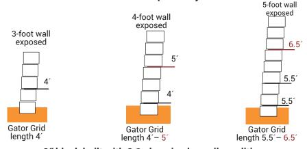
8" block built with 3:1 slope in clay soil condition
