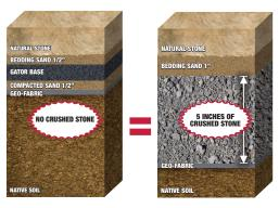
\*The pavers' or natural stones' height (1 1/8 in to 3 1/8 in [2.8 to 8 cm]) will determine the total excavation depth.
