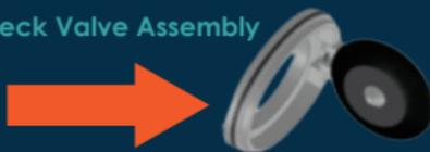
Check Valve Will Be Captured Between Two Pipes
