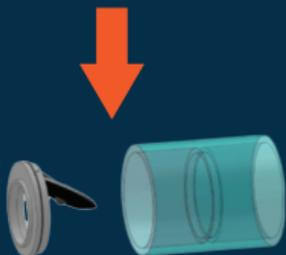
Wet the "O" ring with water for easier installation
