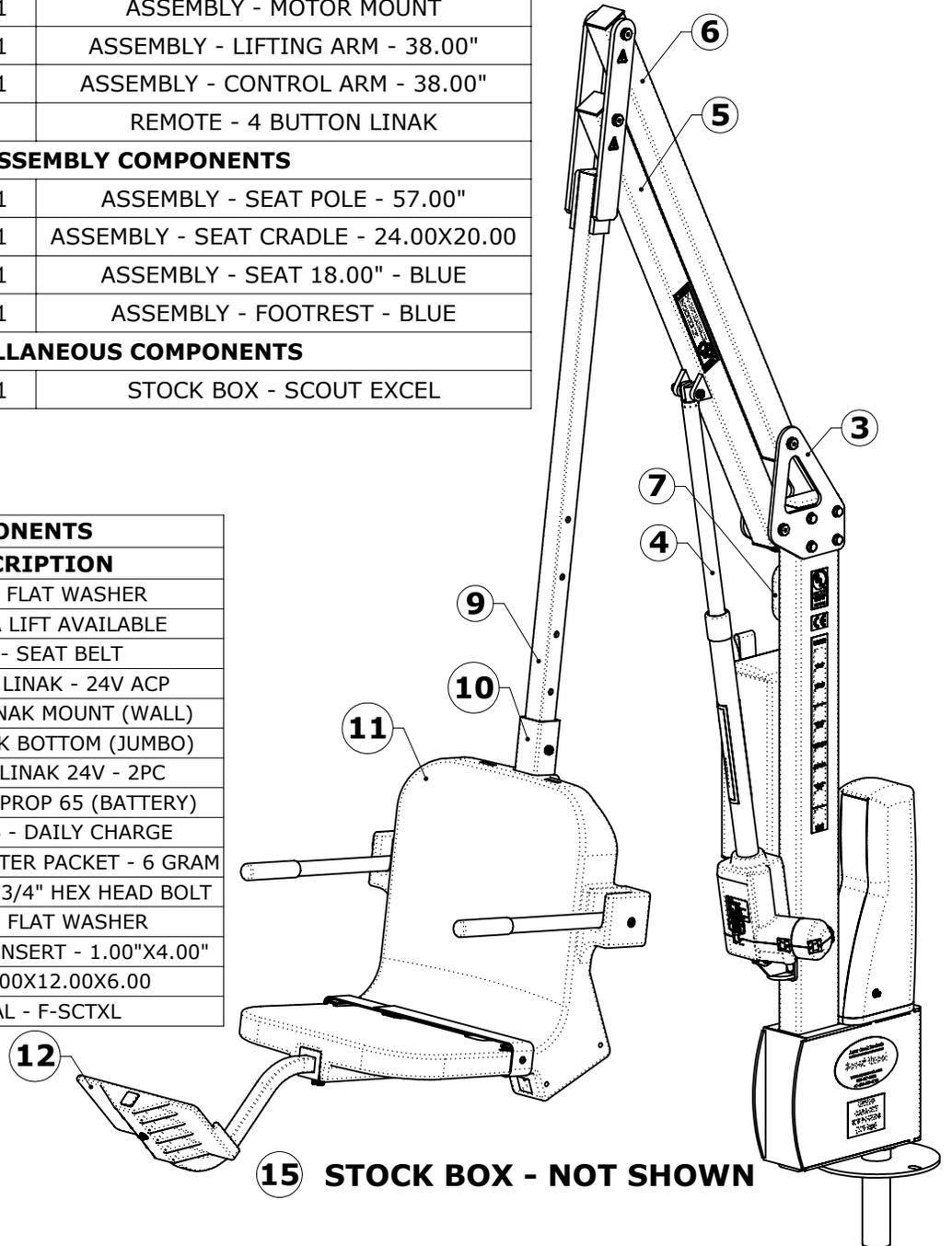
**1** LIFT THE SCOUT EXCEL MAST ASSEMBLY FROM THE SHIPPING CONTAINER. INSERT THE 1.90" [48mm] POST OF THE MAST ASSEMBLY INTO THE DECK ANCHOR. EASE THE MAST ASSEMBLY DOWN UNTIL IT RESTS ON THE DECK SURFACE. ROTATE THE BASE UNTIL THE FIXING ANCHOR HOLE LINES UP WITH THE FIXING ANCHOR. INSTALL THE 1/2"-13X1 1/2" HEX BOLT AND WASHER (PROVIDED IN THE STOCK BOX) TO HOLD DOWN THE LIFT. TIGHTEN THE BOLT.
