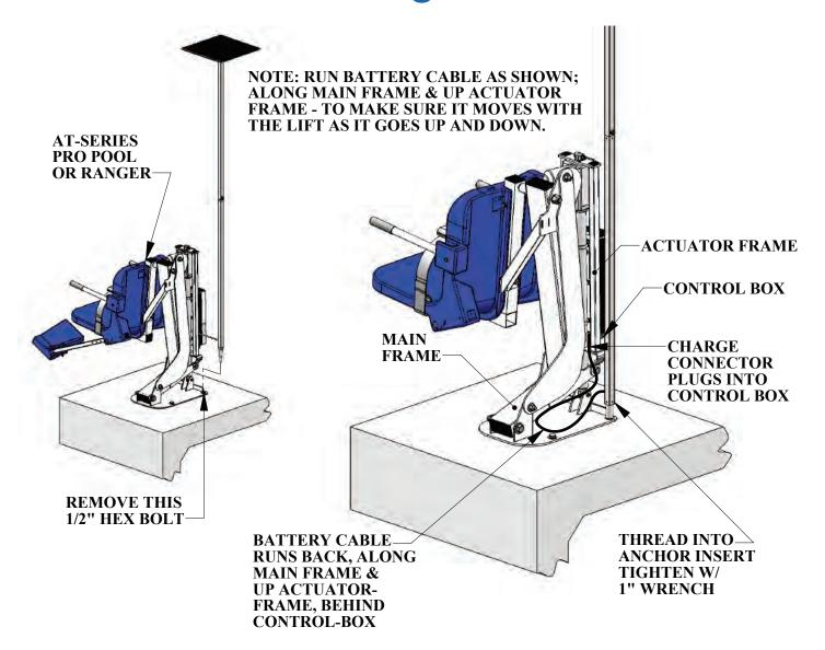
To install the Solar Charger on a Pro Pool-AT or Ranger-AT lift;
