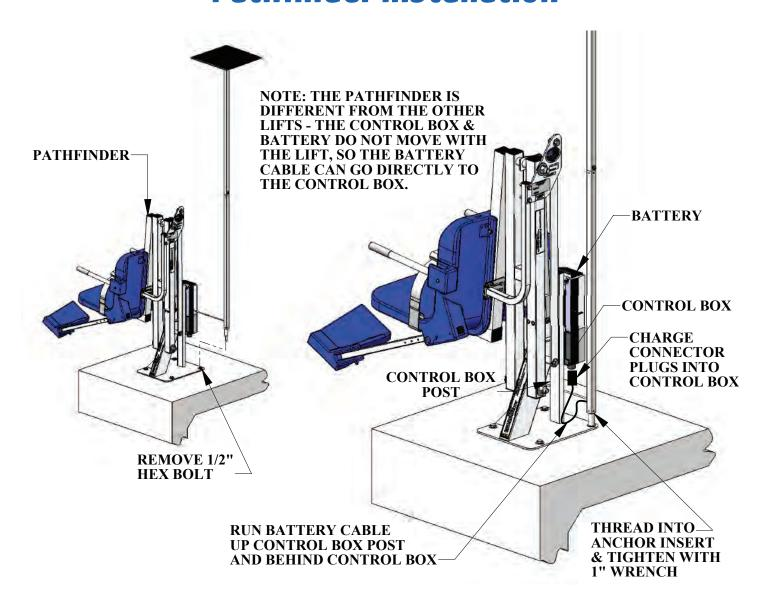
To install the Solar Charger on a Pathfinder lift.
