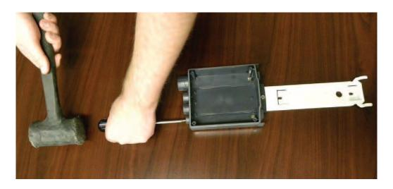
USE SCREWDRIVER, AND MALLET IF NECESSARY, TO PUNCH-OUT AND REMOVE PLASTIC-DISC ON 24V INPUT/OUTPUT PORT
