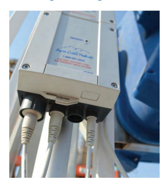
STEP 5: Run the BATTERY CABLE behind the control box as shown, and plug the BATTERY CONNECTOR into the control box.
