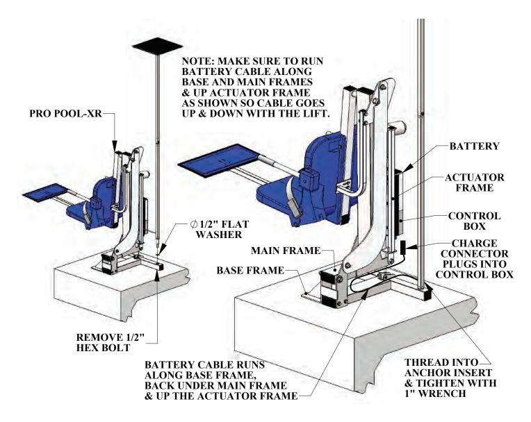
To install the Solar Charger on a Pro Pool-XR lift;
