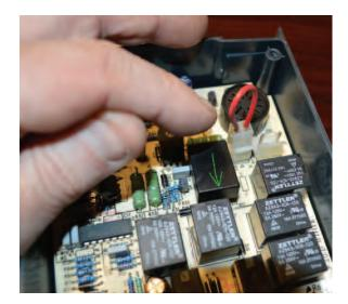
REPLACE THE EMERGENCY-SWITCH CAP WITH "ARROW" POINTING DOWN AS SHOWN
