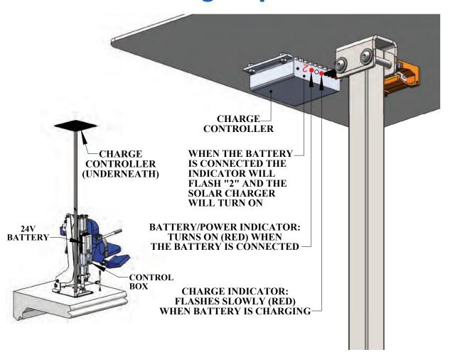
Once the BATTERY CONNECTOR has been installed, and a battery is installed onto the lift the 24V Solar Charger will turn on and start trickle-charging the battery. Without the battery installed the 24V Solar Charger will be off, and will remain off until a battery is installed.
