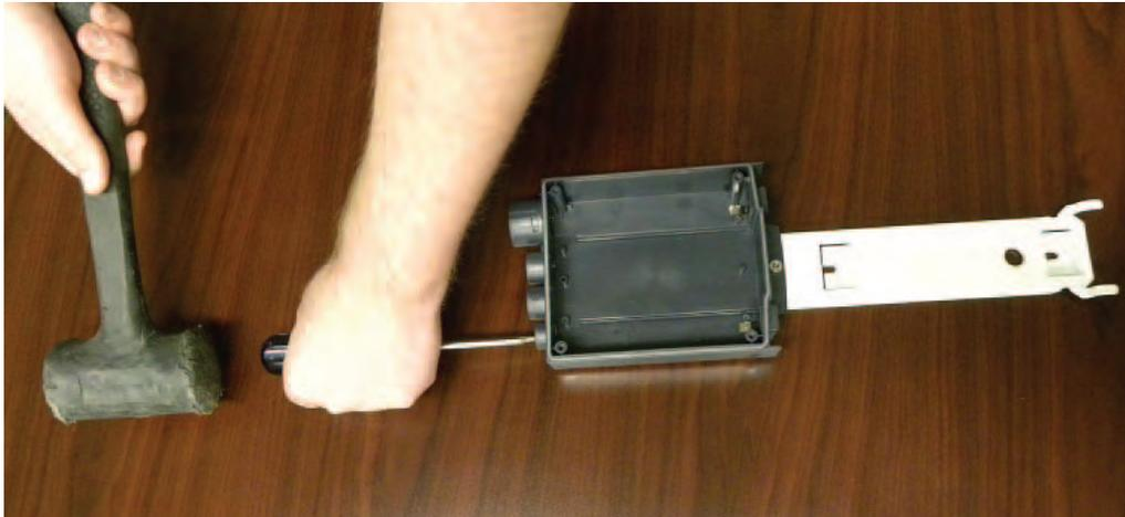
**USE SCREWDRIVER, AND MALLETT IF NECESSARY, TO PUNCH-OUT
