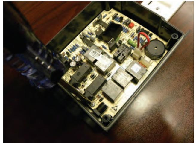
USE A "TORX" T10 DRIVER TO REMOVE THE THREE (3) SCREWS FROM THE CONTROL BOARD
