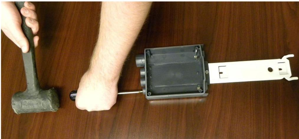
**USE SCREWDRIVER, AND MALLET IF NECESSARY, TO PUNCH-OUT
