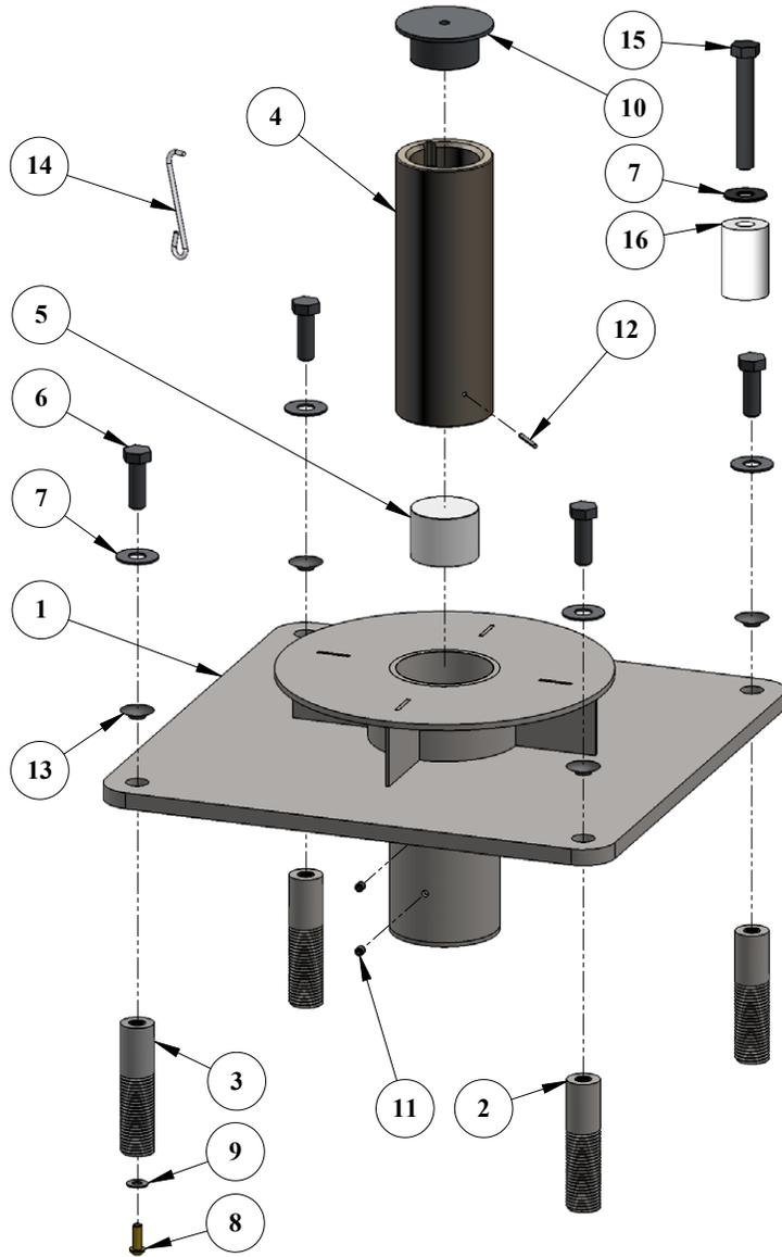
**NOTE:** Item numbers 15 & 16 are for use with the fixing kit attached to the lift. If the anchor was pre-ordered, DO NOT throw these parts away. See page 7 for lift installation instructions.
