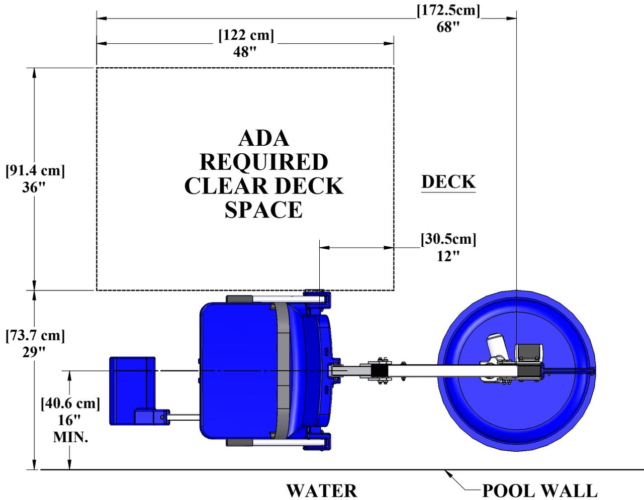
Before installing the Revolution Lift it will be necessary to select a location for the anchor. The Revolution Lifts versatility allows it to be installed in a wide variety of locations, but the owner/installer should be aware of the requirements of the Americans with Disabilities Act (ADA) with concern to lift installations. The diagram above shows an example of an ADA compliant installation, which incorporates the following ADA rules in order to be compliant;
