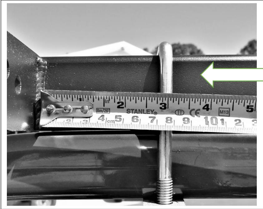
Before mounting the crossbar measure 3" from the inner wall of the crossbar to locate U Bolts.
