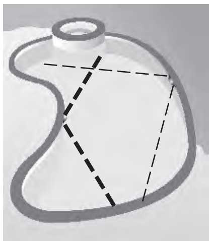
WIDE ANGLE LIGHT BEAM (FOR SIDES OF POOL)
