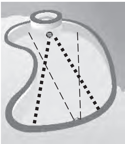
NARROW ANGLE LIGHT BEAM (FOR ENDS OF POOL)
