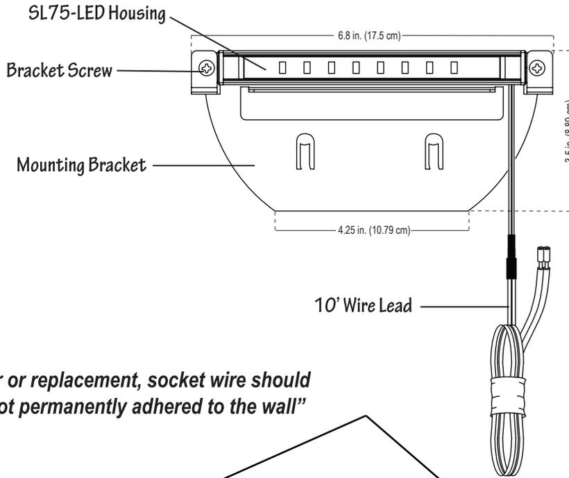
***“To allow for repair or replacement, socket wire should be left loose and not permanently adhered to the wall”***
