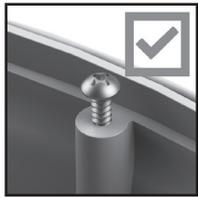
ENSURE AT LEAST THREE THREADS OF ENGAGEMENT AND HAND CHECK BY PULLING EACH SCREW TO ENSURE EACH SCREW IS SECURE
