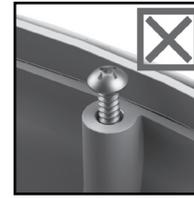
DO NOT USE THE WRONG SIZE SCREWS. IF THE SCREW HOLE IS STRIPPED, BUT NOT CRACKED, A LARGER REPLACEMENT SCREW MAY BE USED
