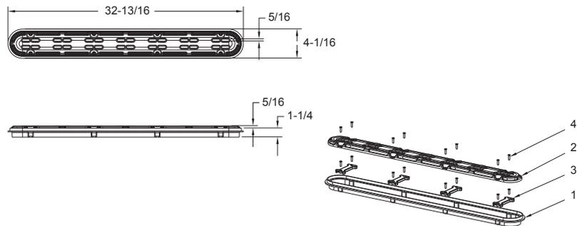
1. 32" channel drain, no sump, frame
