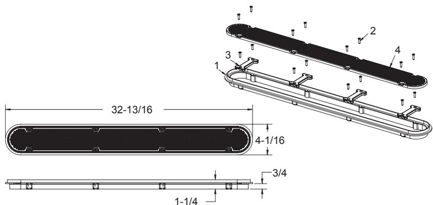
1. 32" channel drain, no sump, frame
