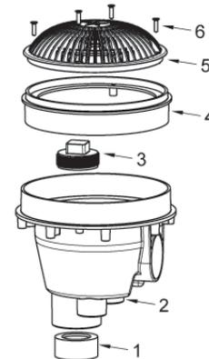
1. 2" Socket x 1-1/2" Socket Pipe Reducer
