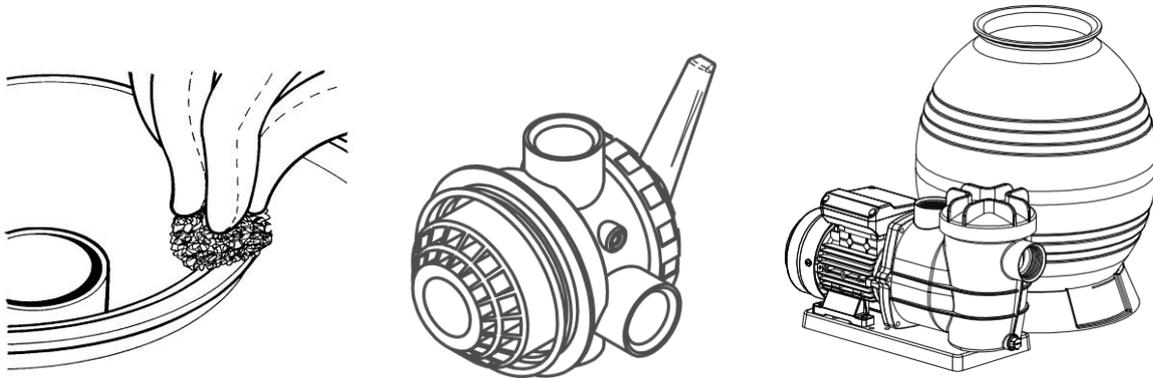
6. Connect the sand tank to pump with hose, hose clamps and hose adaptors.
