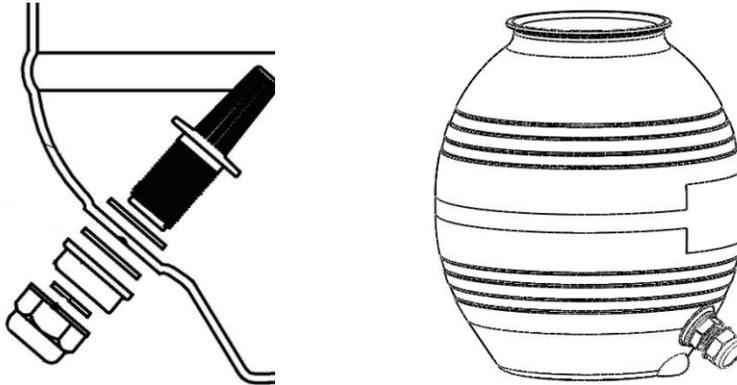
3. Press and turn the sand tank to mount it to sand filter support with correction direction (drain plug is at outside as below picture).
