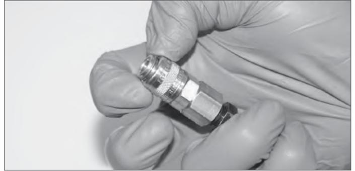
Apply 3-in-1 oil to the Pressure Supply Line Quick-Disconnect, then pull the metal sleeve back and release.
