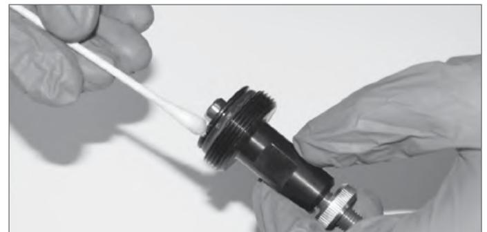
Apply grease to Back Housing Plug Seal.
