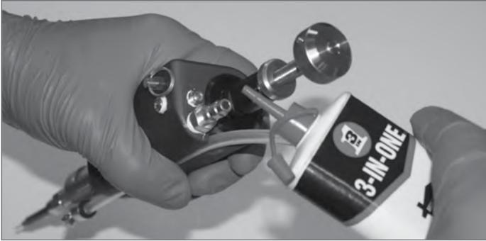
Add a few drops of 3-in-1 oil to the device Pressure Inlet on the injector.
