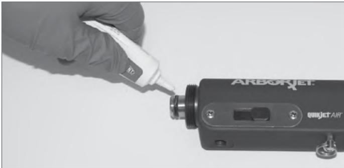
Apply grease to o-ring on Piston.
