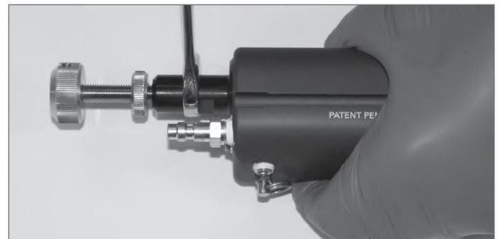
Using a 1/2" wrench, unscrew the black housing plug from body by turning it counter-clockwise.
