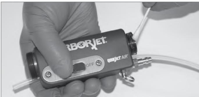
Apply grease to Internal Piston Sleeve
