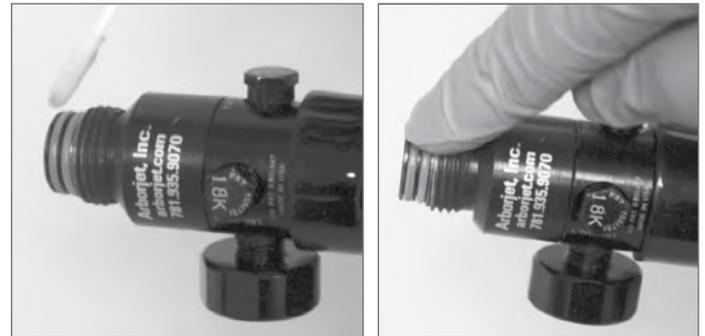
Whenever changing pressure supply tanks, apply grease to o-ring on supply bottle's neck.
