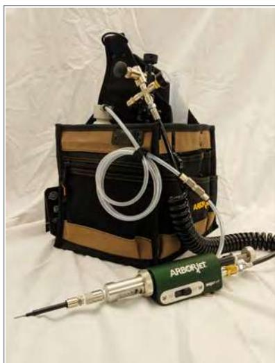
System is assembled, pressurized, primed, and ready for micro-injection.
