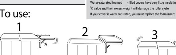
Lock each of the 2 roller racks into position by rotating counter-clockwise, then securing the bottom edge (A) of the brace. Note : Do not bend the roller rack arm more than 90° upward, or damage to the joint may result.
