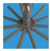
The Aster Series filter utilizes 1" laterals made from injected molded polypropylene. Each lateral is slotted 360 degrees to provide superior filtration and a quick complete backwash cycle.
