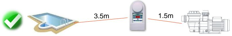
Unit must be 3.5m from pool zone Less than 1.5m from the pump
