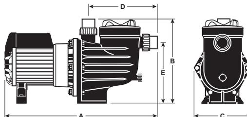
\* Suction and delivery accept 40mm PVC pipe on the I.D. and 50mm fitting on the O.D.
