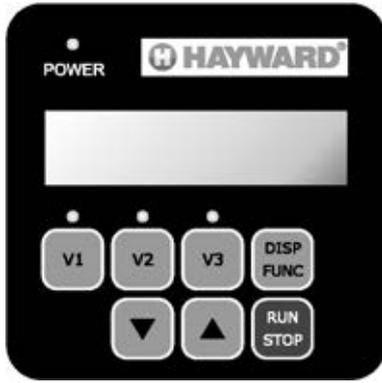
The User Interface is equipped with a membrane keyboard and a digital display with five 7-segment digits.
