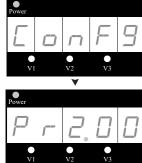
**Press and hold the DISP/FUNC** button for several seconds until the ConFg screen appears.
