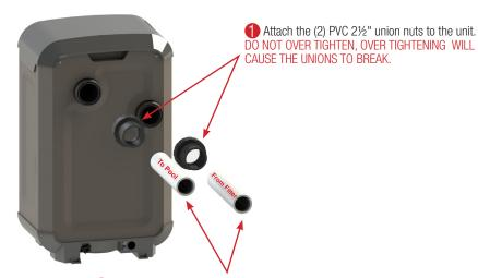
After cutting pipes to length, debur all cut pipe to ensure shavings don't plug critical points internal to the unit. Use PVC solvent cement to glue pipes into the union sleeve. NOTE the inlet and outlet pipe positions.
