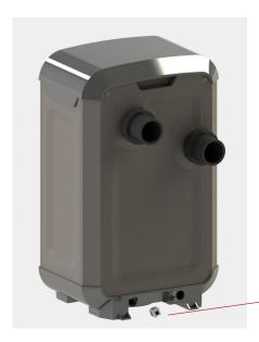
Remove Winterizing O-ring plug near the bottom of the unit by turning counter clockwise. Note, there will be an initial rush of water from the unit after the plug is removed. Allow unit to completely drain, this will take 1-2 minutes. Re-install O-ring plug hand tight.
