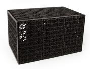
9. To complete the assembly, rotate the Eco-Blox so that the bottom panel is flat on the ground and the top panel is facing up. In this position, the top panel is supported by the sides as well as the center support panels. EcoBlox must always be installed in this position. Improper installation will reduce the structural integrity of the unit and may cause the Eco-Blox to fail.
