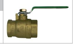
A.Y. MºDonald Mfg. Co. Gas Ball Valves are constructed of heavy duty forged brass. They are designed for residential, commercial, and industrial use in low pressure gas applications. Valves listed are suitable for use with natural, manufactured, mixed and LP gases and with LP gas - air mixtures.
