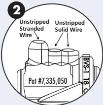
2. Insert unstripped wires into holes. Push wires to back of the connector (wire ends should be visible through clear back of connector).
