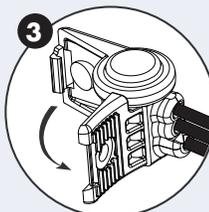
3. Hold wires in place while squeezing handles together until the connector snaps shut.
