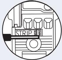
2. Rotate handles fully apart beyond 90 degrees. Insert stripped wires into connector; #12-#14 in the large holes and #16-#20 in the small hole. Exposed ends of wires should be visible through the clear housing on the back.
