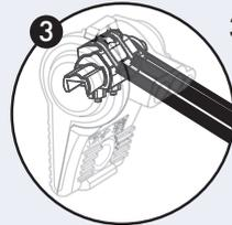
3. Hold wires in place while squeezing handles together until the latch snaps shut.
