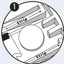
1. Strip wires to 11/16". Use one of the strip guides molded into the connector for reference. Pre-twist stranded wires.
