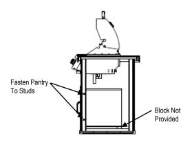
NOTE: Support the back end of your pantry insert with a 1 ¼" x 2 ½" x 38" block. Too much weight inside the pantry insert will cause it to bow and bend. Block NOT provided.
