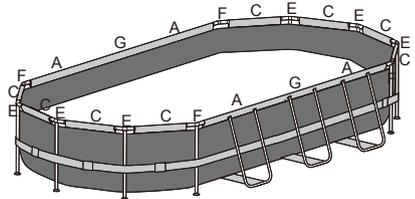
**NOTE:** The installation drawing for the Top Rail and the T-Connector of 24 ft. x 12 ft. x 48 in. (7.32 m x 3.66 m x 1.22 m).
