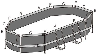
**NOTE:** The installation drawing for the Top Rail and the T-Connector of 10 ft. x 6 ft. 7 in. x 33 in. (3.05 m x 2.00 m x 84 cm).
