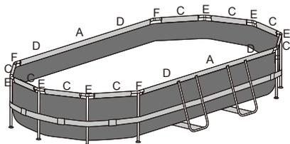
**NOTE:** The installation drawing for the Top Rail and the T-Connector of 16 ft. x 10 ft. x 42in. (4.88 m x 3.05 m x 1.07 m).
