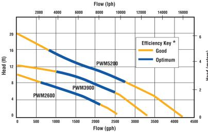
(PWM-Series Pump) Head-Capacity Curves
