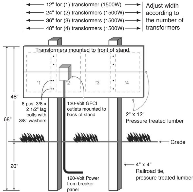
Fig. 8. Transformer Stand Assembly
