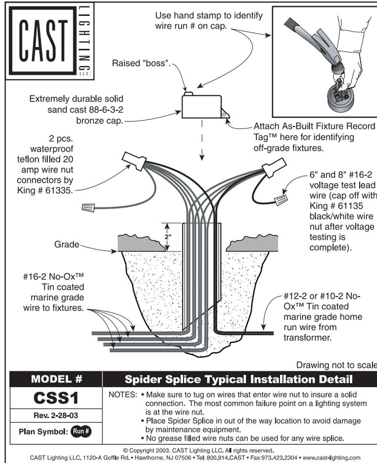
Fig. 5. CAST Spider Splice® connections.
