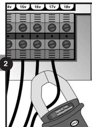
Fig. 19. Amping the voltage taps.
