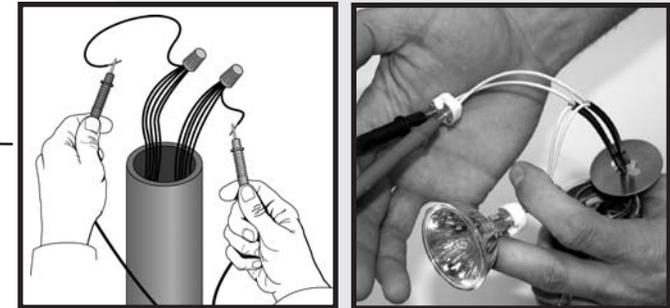
Fig. 11. Testing the voltage at the Spider Splice® or directly at the lamp (using the CAST CTESTMR16 or CTESTS8 - for path lights).
