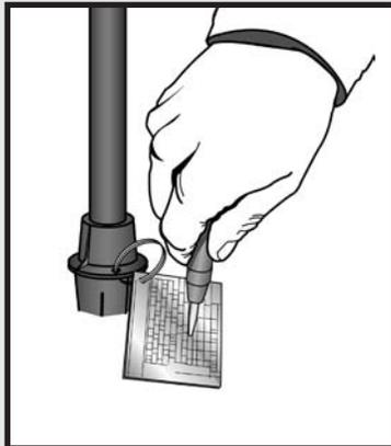
Fig. 22. Marking the Fixture Record Tag with the CAST Center Punch Marking Tool (Model# CPUNCH). Place tag on a scrap of wood when marking.
