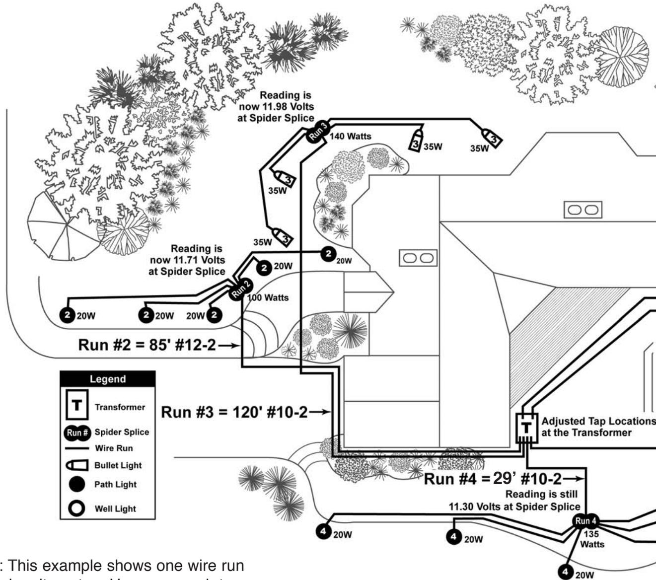
Note: This example shows one wire run to each voltage tap. However, each tap can accommodate up to seven #10 wires or 125 amps/1500 watts.
