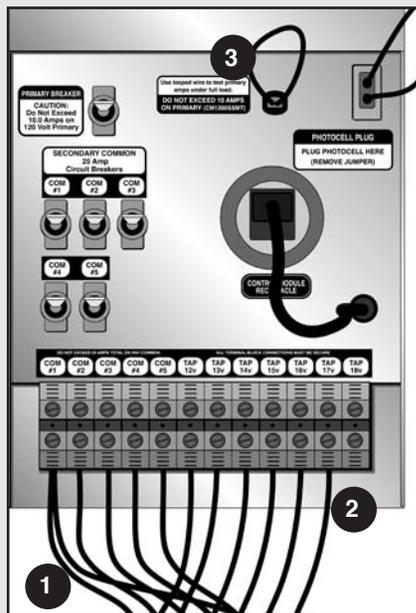
Fig. 17. Final wiring of transformer with test points indicated.
