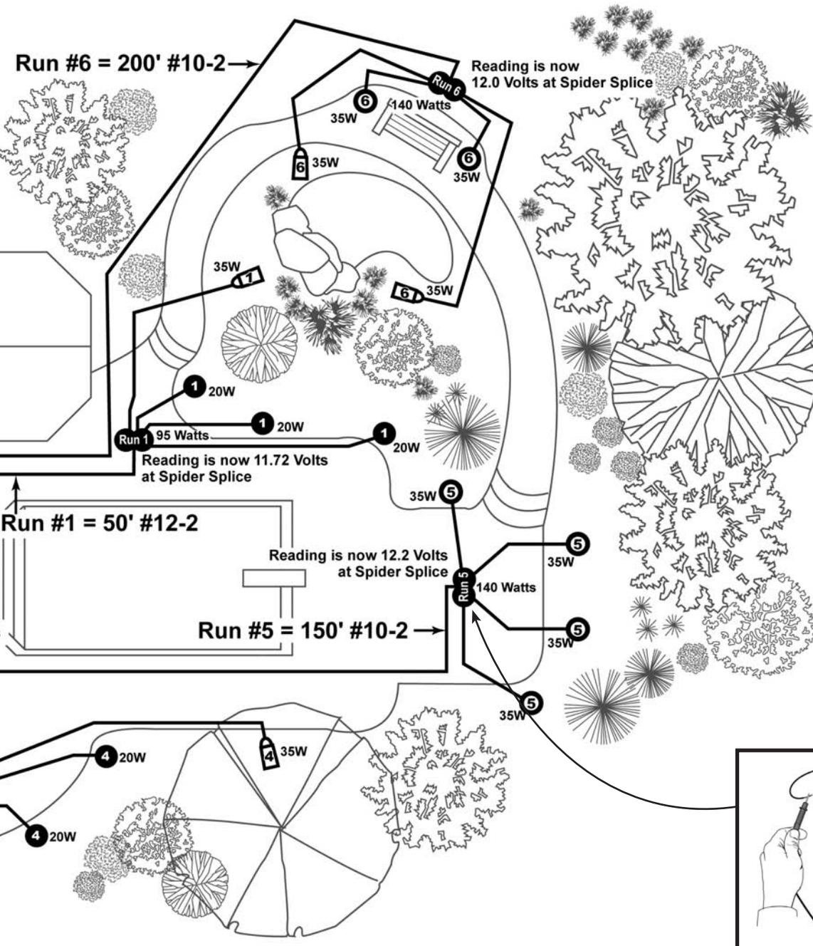
Fig. 15. Retest Voltage at all Spider Splice connections or directly at the lamp.
