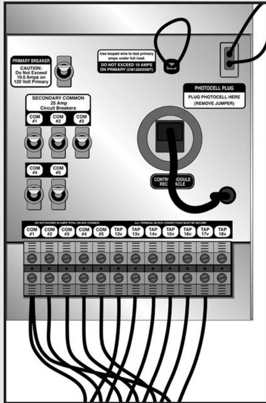
Fig. 13. Transformer with wire runs connected to their appropriate taps.
