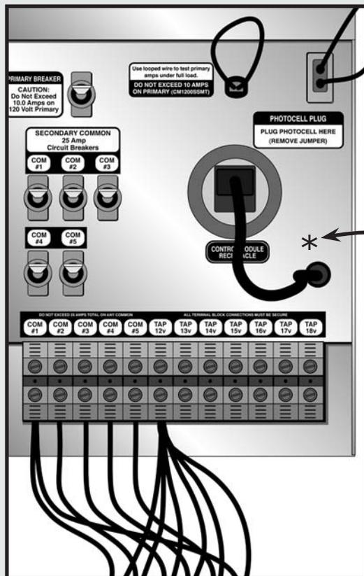
Fig. 9. Transformer with all runs connected to the 12 volt tap. (CAST Model # CM1200SSMT)
