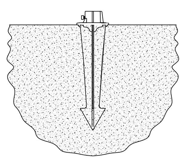
**STEP 1: Install Set-n-Stake ground mount stake.**
