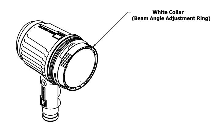
STEP 6: Set desired beam angle by turning the white collar & lining up the black arrow with the desired beam angle indicated on body.
