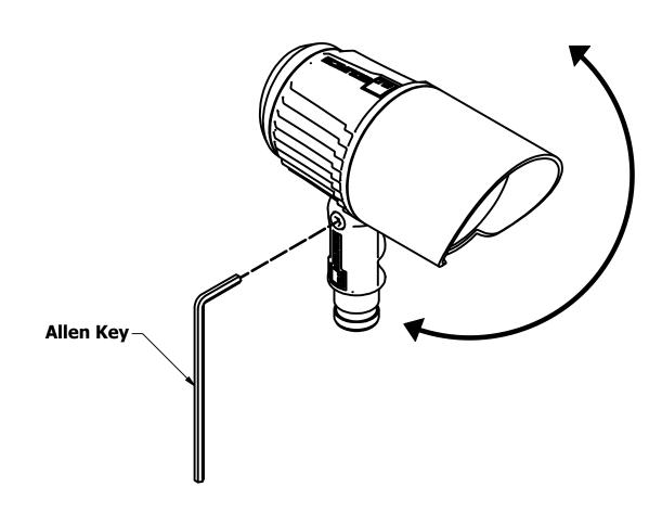
**STEP 4:** Loosen knuckle again with allen key provided & aim in desired direction.
