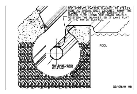
16. After final positioning of the blanket, it must be trimmed to fit the pool contour. A "tongue" should be left where the blanket rises to the surface of the deck to enter the housing. Finally, a draw strap and three button fasteners are included with your solar blanket system.
