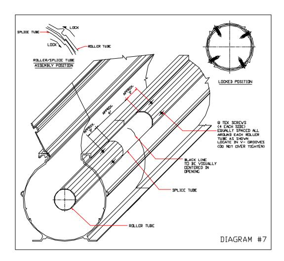
14. To permanently attach the splice tube to each of the roller tubes, use 8 tek screws (4 per side) supplied in the parts bag. Equi-space the screws around the roller tubes approximately 3" from the spliced end. See Diagram #7. Once the splice tube is secured, remove the remaining foam inserts and any debris that may damage the unit or solar blanket during operation.
