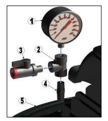
Once the system is started, open vent valve (3) to bleed any air that might have been trapped in the filter during startup.
