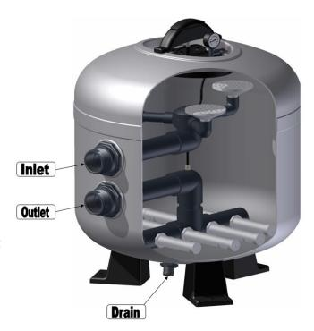
sand bed depth, characteristics of the sand such as granular size, density, etc. A most important parameter is the water filtration rate. Other factors affecting the selection of a filter are the materials used for its construction, the working temperature, and the operating pressure.
