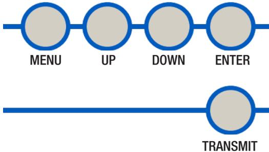
**MENU:** Used to enter menu mode and to navigate back within the menu structure.
