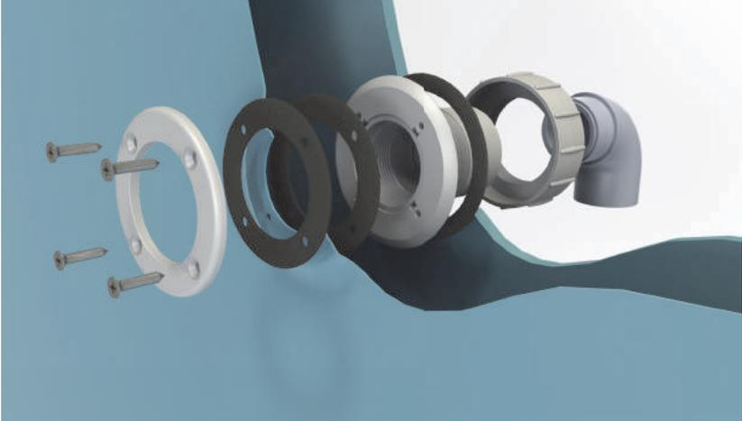
The wall through is connected on the rear to a pipe with a 1,5" threaded coupling.
