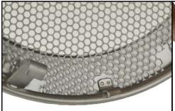
4. Place the bottom of the screen into the face ring aligning the feet around the tab. Note that the smooth beveled side of the screen should face outward toward the front of the face ring.
