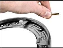
2. Remove the screw from the face ring. Save the screw.
