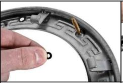
1. Carefully remove the rubber ring from face ring screw. Save the rubber ring.
