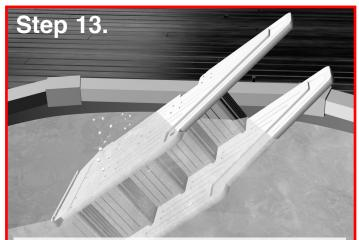
Tilt the unit to allow the steps to fill with water. When bubbling ceases, steps are filled. Steps must be filled completely to prevent floating.
