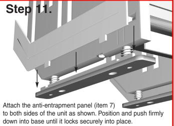
Note: Anti-Entrapment panels are not needed if the unit is left at 48".
