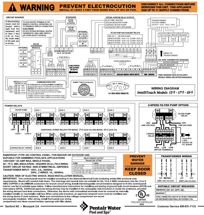
Load Center System Wiring Diagram
