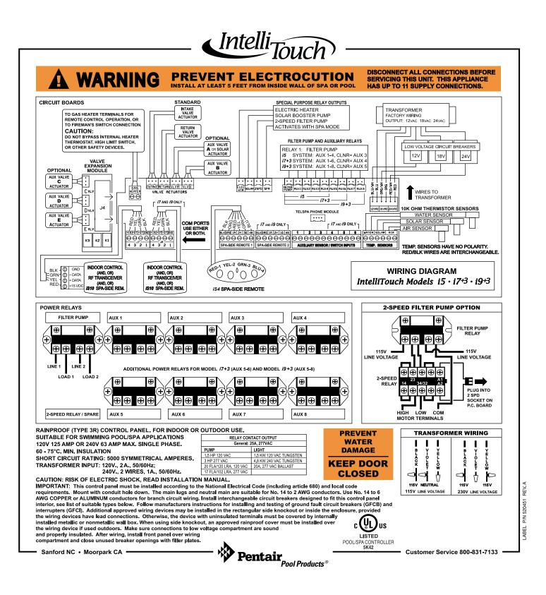
Power Center System Wiring Diagram
