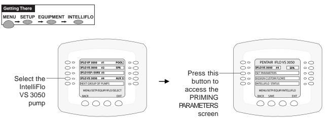
To set the IntelliFlo VS 3050 priming parameters:
