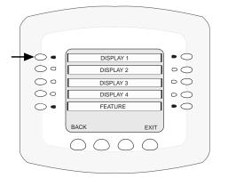
**Display #1** - This screen shows circuit names for the filter pump, pool and spa modes, and all high voltage auxiliary circuits connected to the main Load Center or Power Center.
