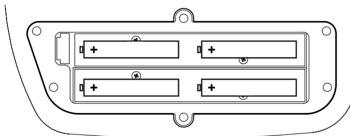
3. Install the battery cover and secure with the six screws. Make sure that the battery cover is secure and that all the screws are hand tightened. **CAUTION - DO NOT OVER TIGHTEN THE SCREWS. OVER TIGHTENING THE SCREWS CAN DAMAGE THE UNIT.**
