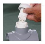
The saddle series sensors utilize the same flow sensor insert used in the tee series sensors
