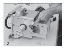
Roll the motor end on it's side. Install the feet on the mechanism using the carriage bolts (36) and nylock nuts (40) provided. Install the feet so the top of the mechanism will be flush with the top of the encapsulation.
