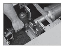
Anchor the non-motor and motor end feet into the housing using as many anchor points as possible.
