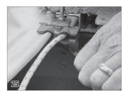
Place the guide retainer (23) underneath the guide feed and onto the screw that goes through the guide feed. Hold the guide retainer flat against the wall of the housing while securing it to the guide feed using a 10-32 nylock nut (29).
