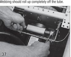
**Adjusting The Torque Limiter**
