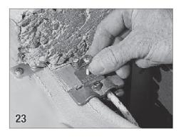
Place a guide feed over the end of the guide, place a bonding lug (25) on top of the guide feed. Insert a  $10-32 \times 1 \, 3/4$ " screw (42) through the lug and guide feed.
