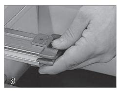
Using a 5/32" allen wrench, loosen the screw on the top of the guide feed (16). Insert the guide feed on the end of the guide that will extend into the housing.
