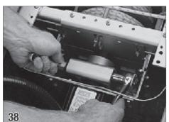
To adjust the torque limiter, use two 1/2" wrenches to tighten one nut and bolt 1/2 turn. Rotate the torque limiter 180 degrees and tighten the other bolt and nut 1/2 turn.
