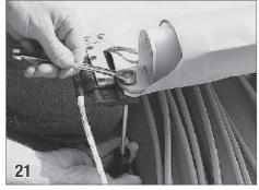
Secure the leading edge insert support bracket to the slider by placing the 10-32 X 1" (41) screw up through the slider, the hole in the front corner of the cover, and through the support bracket. Tighten completely using 10-32 nylock (29), then back the nut off 1/2 turn.
