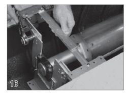
Now loosen the bolts and spread the pulley brackets at the non-motor end making sure they are also level. Raise the pulley bracket so it is flush with the top of the encapsulation. Center the non-motor side front to back in the housing.
