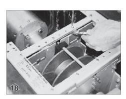
On the motor <u>and</u> non-motor side, use a 3/16" bit and drill throught the cross braces. To secure, use the half inch screws (27) and nylock nuts (29) provided and bolt the cross braces together in two places on each cross bracket.
