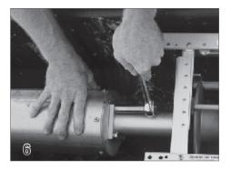
Attach the cone on the motor end using the same bolts (36) and washers (37). Tighten the bolts using a 9/16" wrench.
