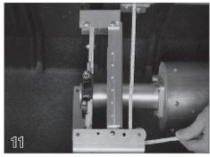
Go to the non-motor end and make sure the rope will come straight back from the guide to the pulley. It is important that the tube is centered between the guides.
