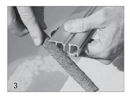
Before splicing the sections of guide together, file all guide ends thoroughly, rounding all edges and removing all burrs. **This step is extremely important!**
