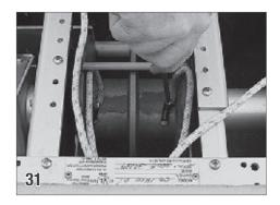
Bring the ropes back to the mechanism. Attach the ropes to the rope reel by placing a  $\#10 \times 1/4$ " pan head screw (33) through the ropes and into the rope reel.
