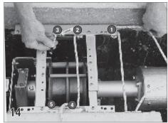
Run the the non-motor end rope behind the motor end rope as it passes behind pulleys #1 and #2 and around pulley #3. Continue pulling the rope to the front side of the mechanism. Run the rope around pulley #5 with the rope coming off the bottom of the pulley. Pull all the excess rope through and lay it on the deck in front of the mechanism.
