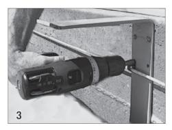
Secure the brackets to the back wall of the housing using #12 x  $1\frac{1}{2}$  "hex head sheet metal screws. Mount a rope loop on one screw of each of the brackets. This will keep the rope running straight along the back of the housing.
