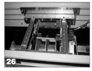
The mechanism mounting plates have threaded holes in them that line up with the mounting holes in the pulley brackets. Insert  $\frac{1}{4}$  -20 x  $\frac{3}{4}$  inch bolts into these holes and secure the motor end of the mechanism to the mounting plates.
