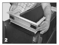
Place the preassembled boxed riser ends (A2410) at each end of the housing.
