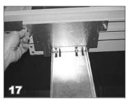
Install  $\frac{1}{4}$  - 20 nylock nuts onto the (2) pem studs in the anchor plates. Do not tighten these nylock nuts down at this time so the mounting brackets can slide side to side to position the mechanism in the correct location.
