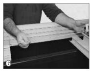
Using the piece of riser that is 40 inches long and notched at each end (M9354), cut the riser to fit on the front side of the housing for the motor and non motor ends. The cover guide will pass through the notches in the riser.
