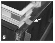
Insert the fixed height hooks (M9356) into the channel on the outside of the riser. These hooks will rest on the housing and set the height of the riser 4 inches above the housing.
