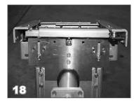
Both, the Eclipse and Aluminum mechanisms are being shipped with the pulley brackets on both the motor end and non motor ends already set at the correct width and height for the *QuickAttach* system.
