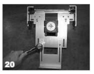
Install the mounting feet on the non motor end of the mechanism. For the Eclipse mechanism, use the top hole to mount the feet. For the aluminum system, use the fifth hole down from the top.
