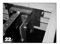
Install the non motor end of the mechanism so the slots in the pulley brackets slide over the pem studs in the mechanism mounting plates.
