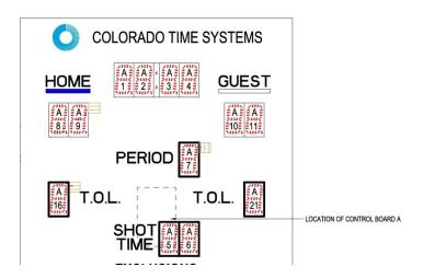
2. Set the Channel and PAN on the dip switches for control board A.
