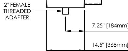
**SUMP AND GRATE:** UNBLOCKABLE SOFA CERTIFIED TO APSP/ANSI/ICC-16 2017, NSF/ANSI/CAN 50-2020, AND USPC. RPD FIELD CERTIFICATION IS NOT REQUIRED. CORROSION RESISTANT, NON-CONDUCTIVE, NON-MAGNETIC, AND REQUIRES NO BONDING.
