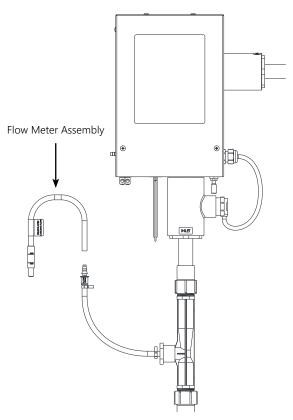
Figure 3: Flow Test Diagram
