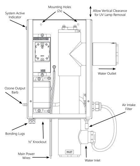
Figure 1: Mounting Location & Notations (cover removed)
