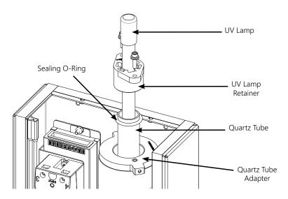
Figure 6: Lamp and Quartz Tube Removal
