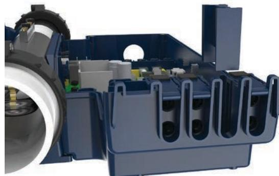
Once all in.claw's and shut-off are reinserted, replace the cover. Cover screws should be tightened to a max of 8 lb.in (0.9 N.m).
