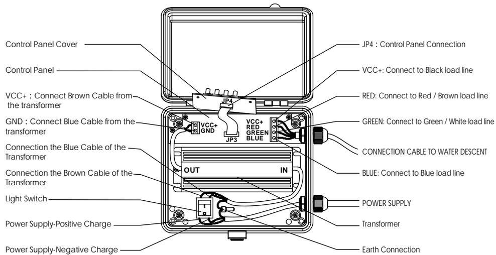
**Warning:** load of the control box should not exceed 60W.
