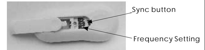
Each control box is associated with a remote control. To use a single remote to control a multiple number of control boxes, you would need to configure the Frequency at the back of the remote control. The Frequency of the Remote would then need to be synced with all the control boxes.
